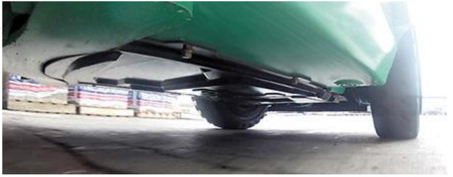
For a forklift truck, that means a belly plate with sealed rear wheel arches. Putting a physical barrier under the truck stops dust and dirt being sucked into the engine and sprayed around – especially if the wheel arches are included. This protection can be fitted to most trucks, and some – like the Mitsubishi [GRENDA](#) – even have it as standard.
